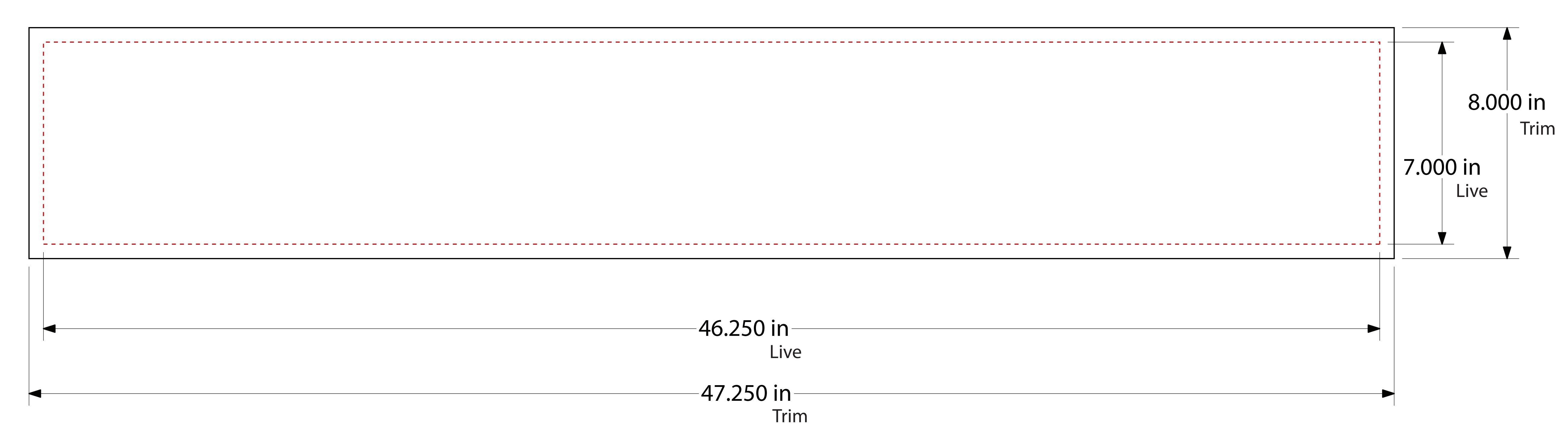
HEADER SUBSTRATE THICKNESS: Recommended minimum 0.070" Thick Clear Polycarbonite including ink or digital decal.
