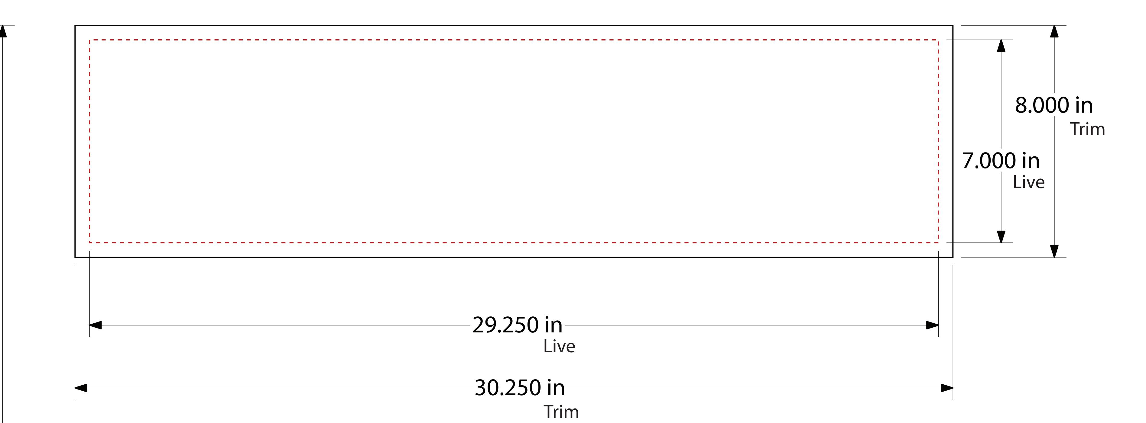
HEADER SUBSTRATE THICKNESS: Recommended minimum 0.070", absolute maximum 0.1875" Thick Clear Polycarbonite including ink or digital decal.
