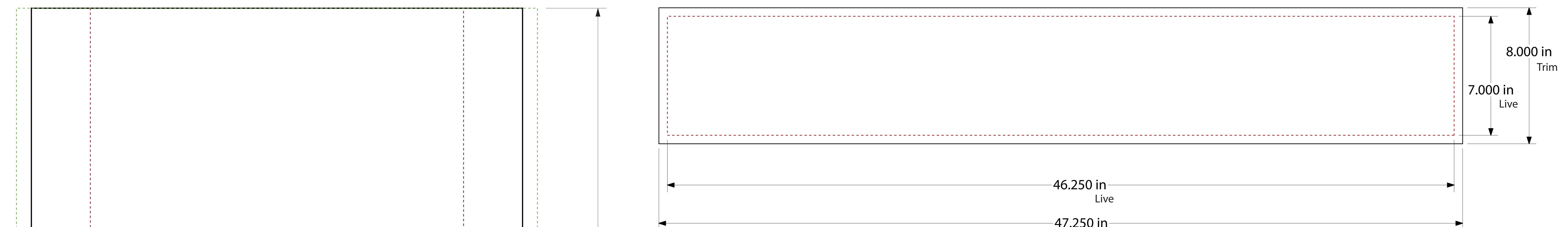
HEADER SUBSTRATE THICKNESS: Recommended minimum 0.070". Clear Polycarbonite including ink or digital decal.
