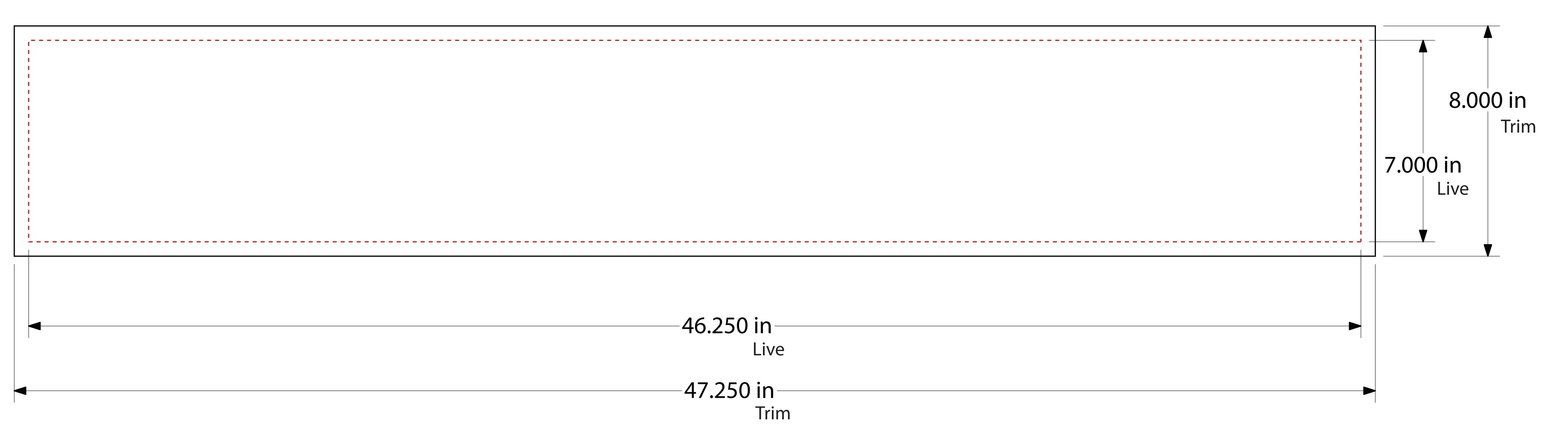
HEADER SUBSTRATE THICKNESS: Recommended minimum 0.070" Thick Clear Polycarbonite including ink or digital decal.
