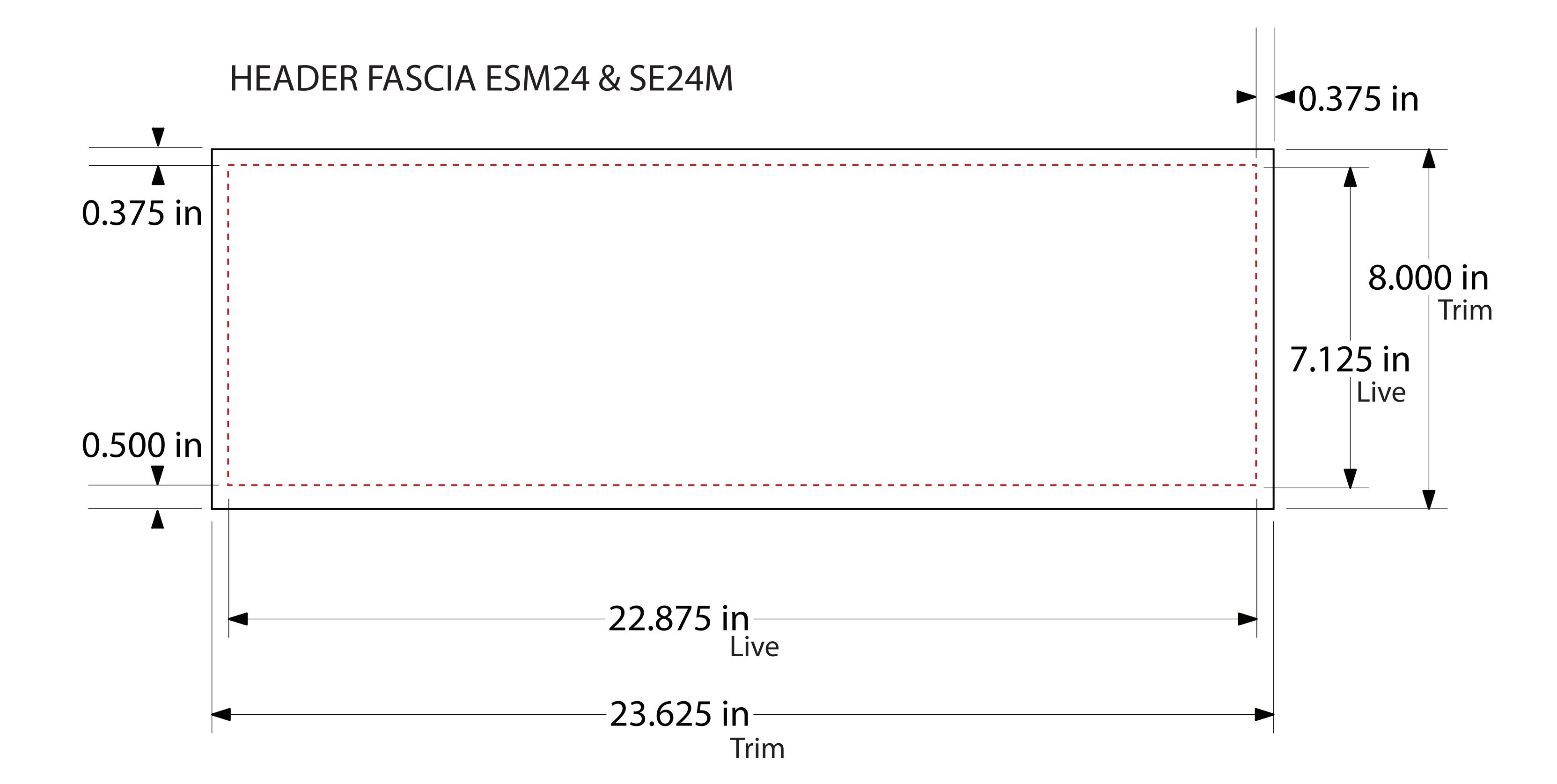
HEADER SUBSTRATE THICKNESS: Recommended minimum 0.070", absolute maximum 0.1875" Thick Clear Polycarbonite including ink or digital decal.
